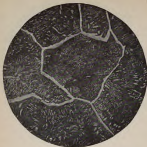
FIG. 12.—CEMENTED BAR, FULLY CONVERTED— STRUCTURE UNIFORM THROUGHOUT— CARBON 1.6%. Magnified 33 diameters.
